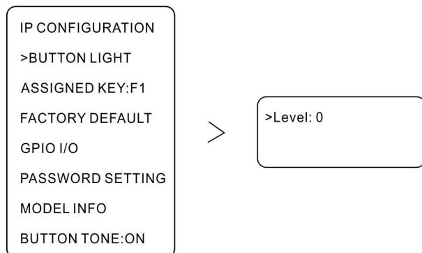
There are 3 modes for controller key lighting: Level 0 (no light), Level 1 (normal light), Level 2 (strong light). The default setting is Level 1.
