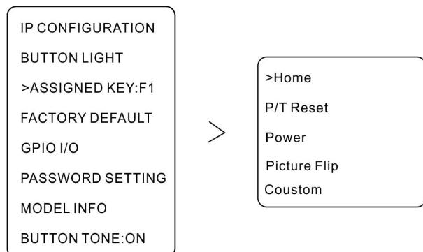
F1 ~ F4 are custom buttons. To customize the button, switch the button by shaking the joystick left and right.
