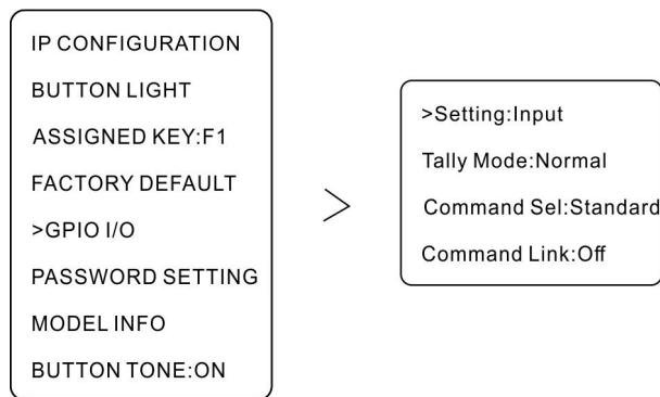
**Setting:** Set the I/O port type: optional Input or Output
