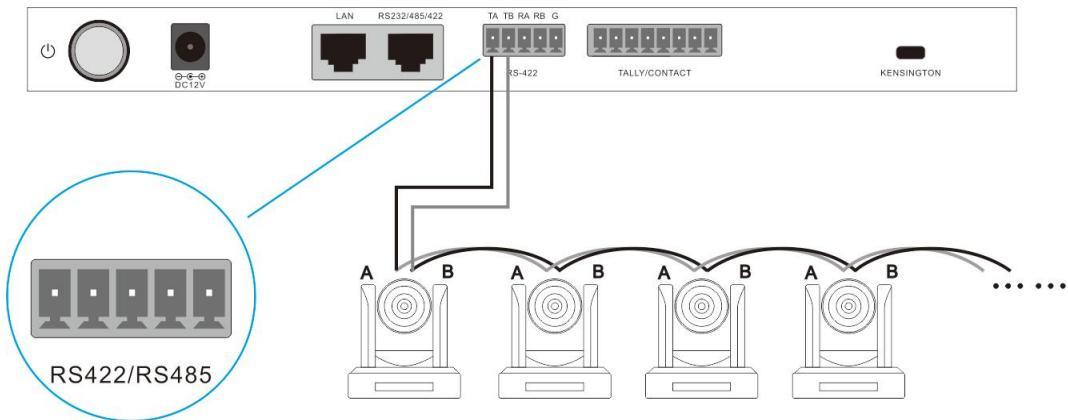
The following table lists the corresponding camera wiring.
