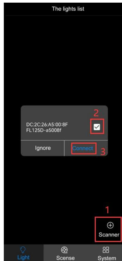
When you need to reconnect after disconnection, click "Light" and select the desired connected device in the light list, click "Connect Device" to connect.
