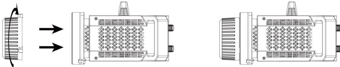
①. When installing the protection cap, align the protective cover with the Bowens mount points, rotate the protective cover, and fasten the protective cover to the lamp body.
