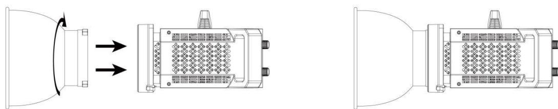
①. When installing the reflector, align the reflector with the Bowens mount points, rotate the reflector, and fasten the reflector to the lamp body.
