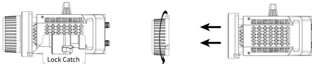
②. When removing the protection cap, press down the lock catch and rotate the protection cap at the same time to take out the protection cap.
