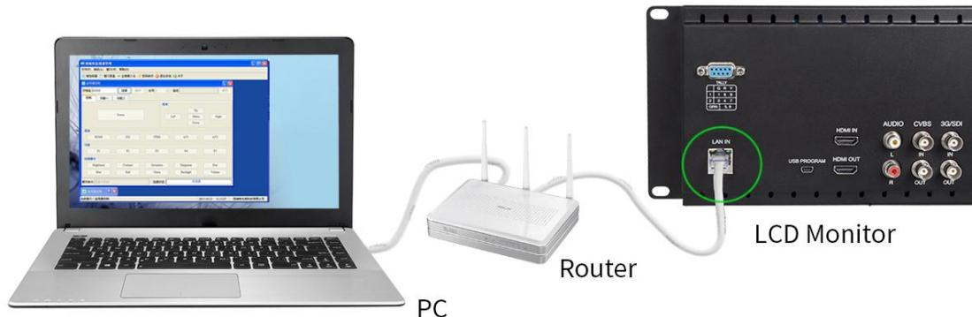
Connect the LAN port on the back of the monitor to the network. After connection, the monitor will display the same IP address with that device.
