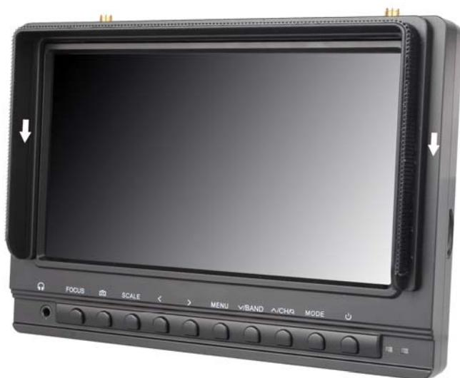
**4.3** Put the corresponding sun shade with paste tape, follow the image and paste on the fixed frame.
