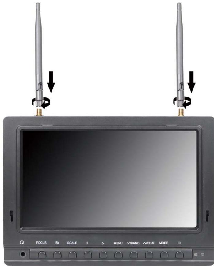
Take the matching antennas assemble on the unit's antenna input ports; the assembly should be secured and locked on the buckle.
