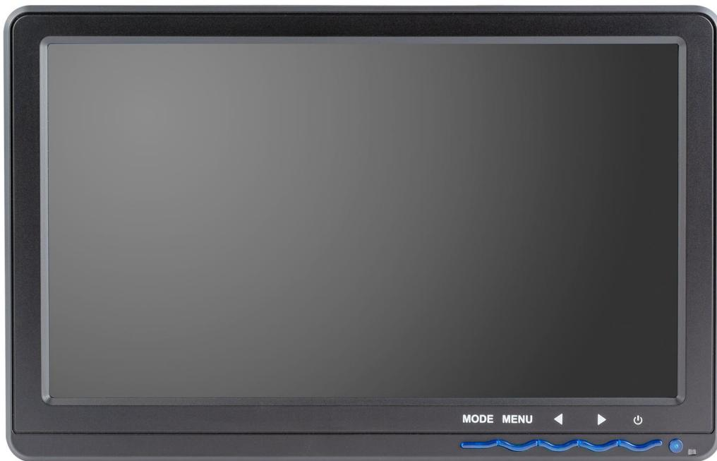
**MODE:** To switch VGA, AV, HDMI input signals
