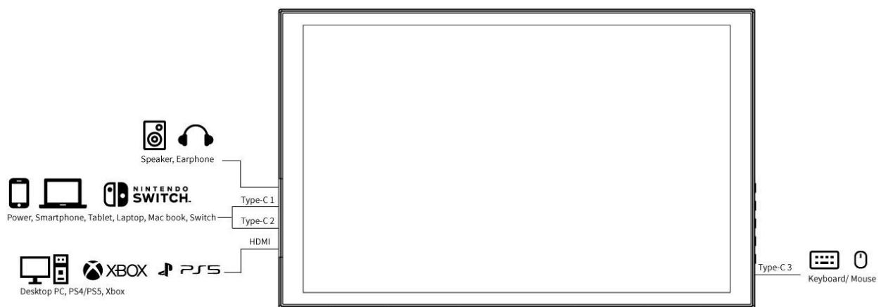
**Note:** Phone for IOS system, MAC notebooks (without HDMI interface) need to use adapter devices, such as Lightning to HDMI cable
